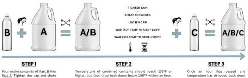
Part A. Tighten the cap and shake for 30 seconds to help begin catalyzation process. After shaking, set the bottle down and loosen the cap to allow vapors to escape. It is imperative to loosen the cap immediately after shaking Parts A & B together. Otherwise, product won't catalyze properly.
